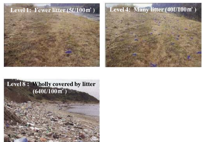
Fig. 1. Example of 'Index Evaluation Measurement of scattered trash'. Blue area of Level 1 and 4 means trash scattered on a beach. The index can be used as an alternative way to rapidly assess beach litter pollution in a wide area. Surveyors can easily assess the pollution level of a beach with the reference photos and estimate the total amount of litter.
