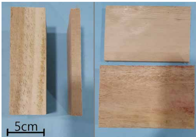
▲ Figure 3. Two sizes of wood drifters are placed on its side (left) and seen from above (right). The measurements of the thick drifter is 15*10*5 cm and 15*10*1.5 cm for thin ones.
