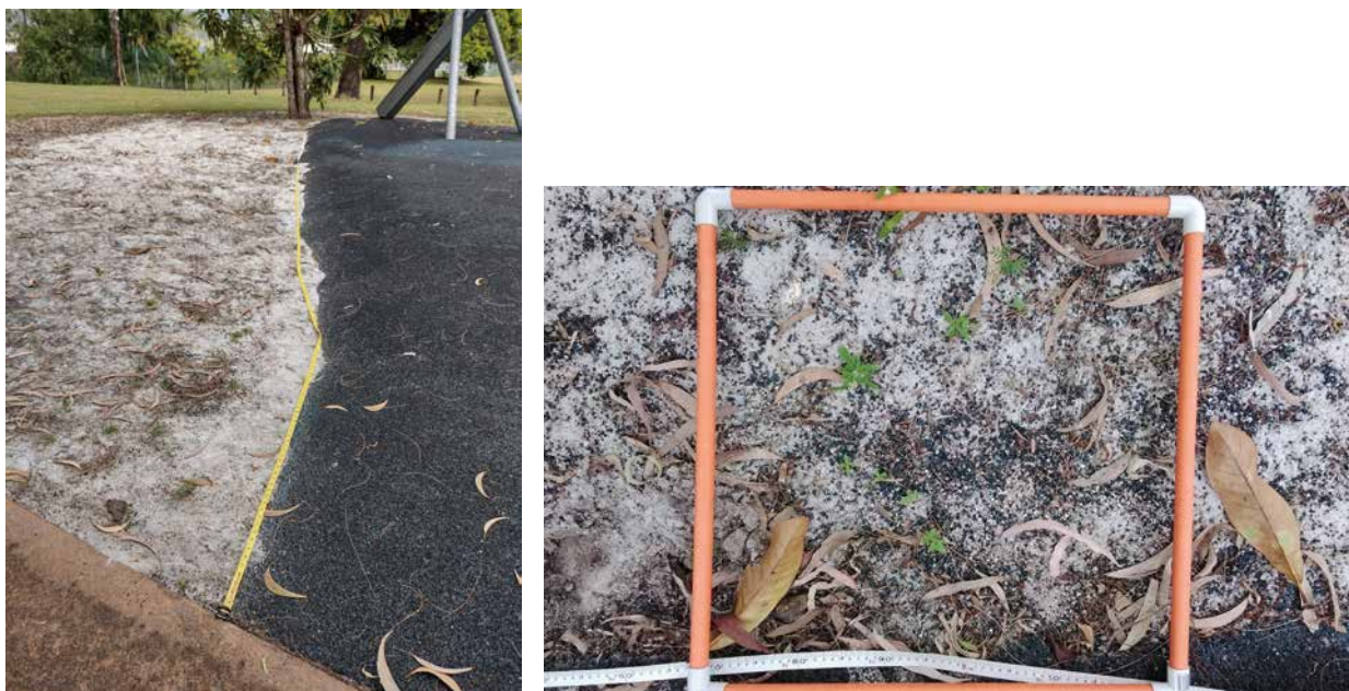
▲ Image 2. A sampling of rubber crumb at the Coral Sea Park playground, Cardwell QLD (Source: ReefClean AUSMAP Rubber Crumb Assessment Report 2021).
