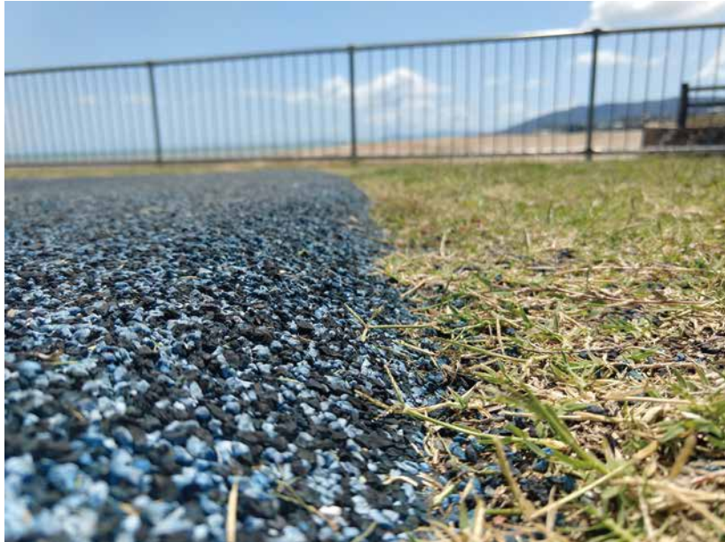
▲ Image 4. Rubber crumb playground matting (Source: ReefClean AUSMAP Rubber Crumb Assessment Report).
