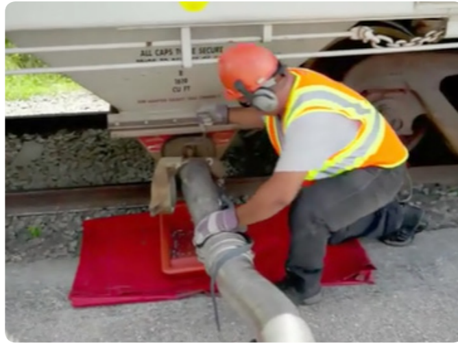
Fig. 6. Using a tarpaulin and catch tray underneath an unloading valve can help to contain any potential pellet spills (TRANSFLO, 2015)
